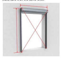
**Step 7**: Fixing the both side of the guide rail (there are reserved fixing holes on the guide rail)
